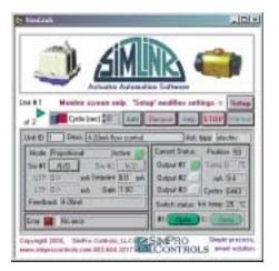
To set up a controller, the setup button in the main screen opens the setup screen. Here, you can select the control mode and associated settings. An optional help list guides you through the
