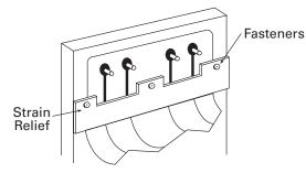
Figure 5-8. Strain bars, screws or clips can be used for circuit mounting.
