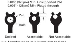
Figure 6-7. Annular rings minimum dimensions.
